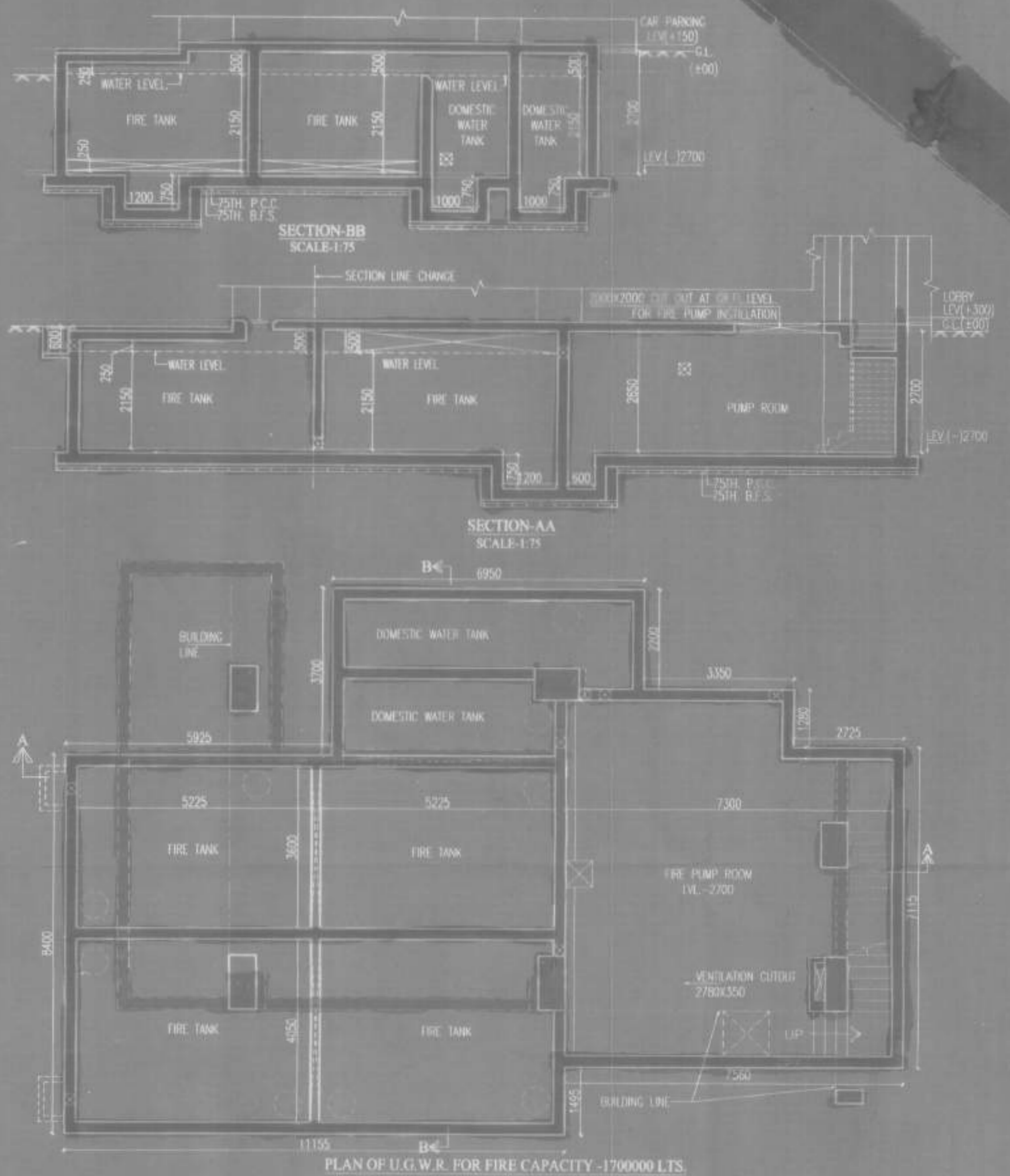
PLAN OF U.G.W.R. FOR FIRE CAPACITY - 1700000 LTS. PLAN OF U.G.W.R. FOR DOMESTIC USAGE CAPACITY - 40000 LTS. PLAN OF FIRE PUMP ROOM (SCALE: 1:15)
